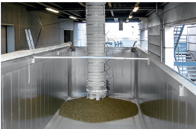
Open loading: as the bulk material cone rises, the discharge automatically lifts.
