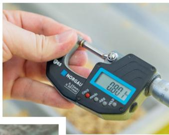
A final quality check of the thickness of an oat flake is carried out in the laboratory.
