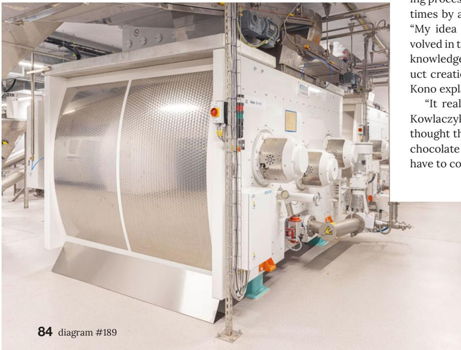
Bühler’s DÜC conches bring flavors to life. With the new process design of the DÜC S conche, Wedel was able to reduce process time by around 30 percent.
