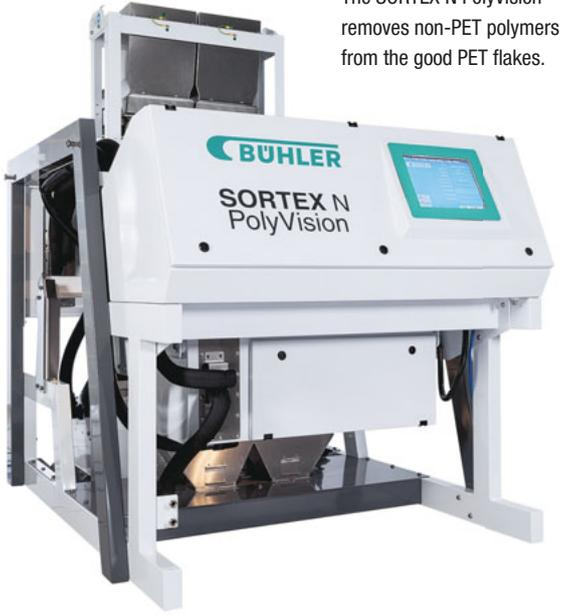
The SORTEX N PolyVision removes non-PET polymers from the good PET flakes.
