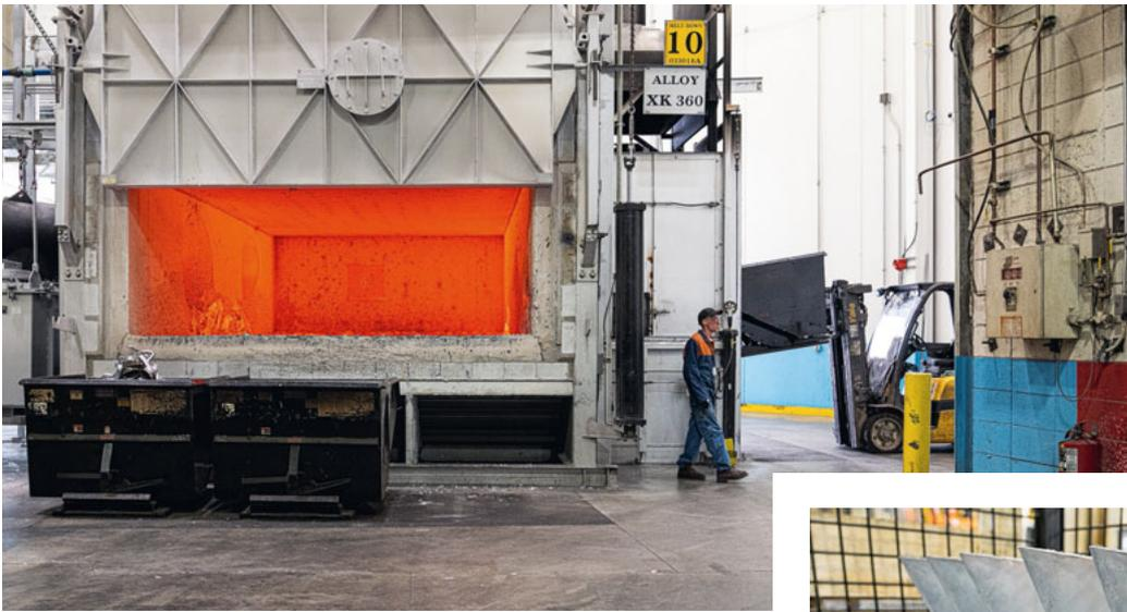
The reverberatory furnace is where the special alloys are produced. The pre-melted and pre-mixed metals and alloys are melted together here.
