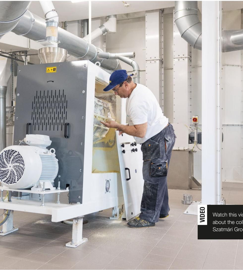
Miller Imre Szabó checks the Pulsroll hullers. They degerminate the maize more smoothly and precisely.
