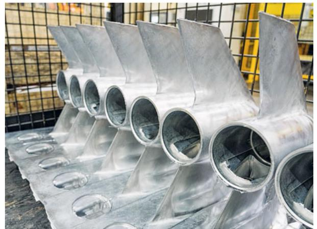
The gear casing is the biggest part that Mercury Marine die casts.
