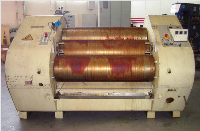
Three-roll mill type SDV 1300 before reconditioning
