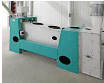
Screening machine GrainPlus LAGA to remove contaminants
