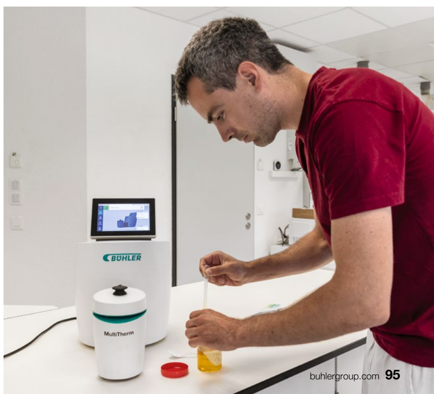
Bühler’s MultiTherm can be used to determine the crystallization property of cocoa mass and cocoa butter, which are important quality criteria in the production of chocolate.
