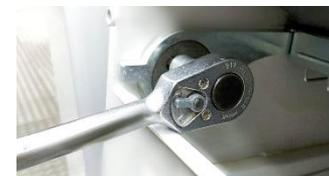
The quick-clamping system enables the sieve layer exchange in less than 5 minutes.
