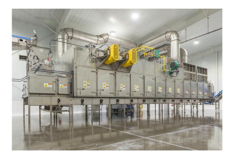
From French fries, slivers and nubbins, to dehydrated potato products and co-products, Bühler's AeroDry conveyor dryer with heavy duty stainless steel construction efficiently processes potatoes for every application imaginable--functioning as an oven, roaster, toaster and cooler.
