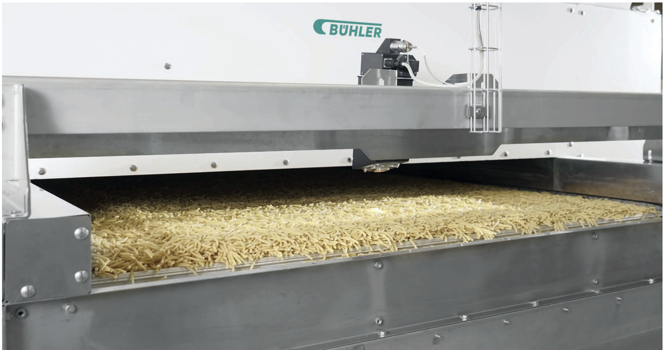
Sensor measuring moisture of short-goods pasta.
