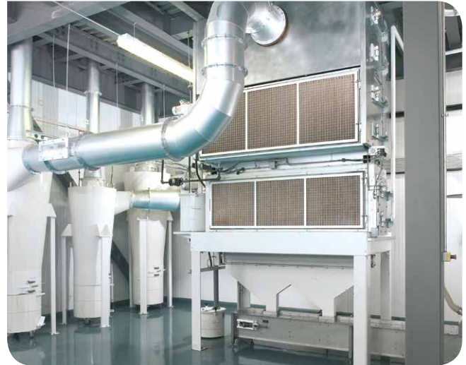
Barh RoaStar vertical roaster with two roasting zones and one cooling zone
