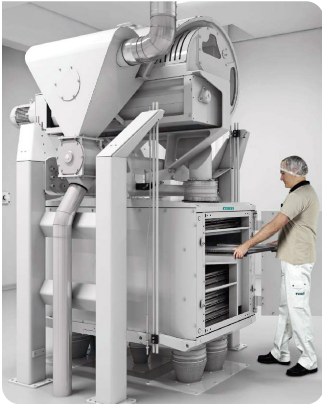
Easy screen frame changes from both sides.
