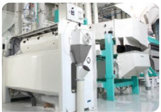
The Application Center offers rice milling machinery starting from pre cleaning, cleaning, hulling, whitener, polisher, grading and finally the sorting of grains based on colour defects using colour sorter machine to offer rice grains which is of high quality & free from defects, foreign particles and even more.
