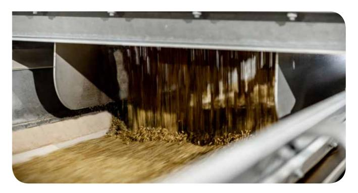
We offer a range of solutions to convey all Our transport systems for wet grain and green products in the malting plant gently between malt feature an integrated washing unit and production steps, including belt conveyors, numerous access points for manual troughed chain conveyors, screw conveyors cleaning, ensuring low-residue transportation. and belt elevators. In order to achieve the highest levels of food safety, our conveyors are made of stainless steel.
