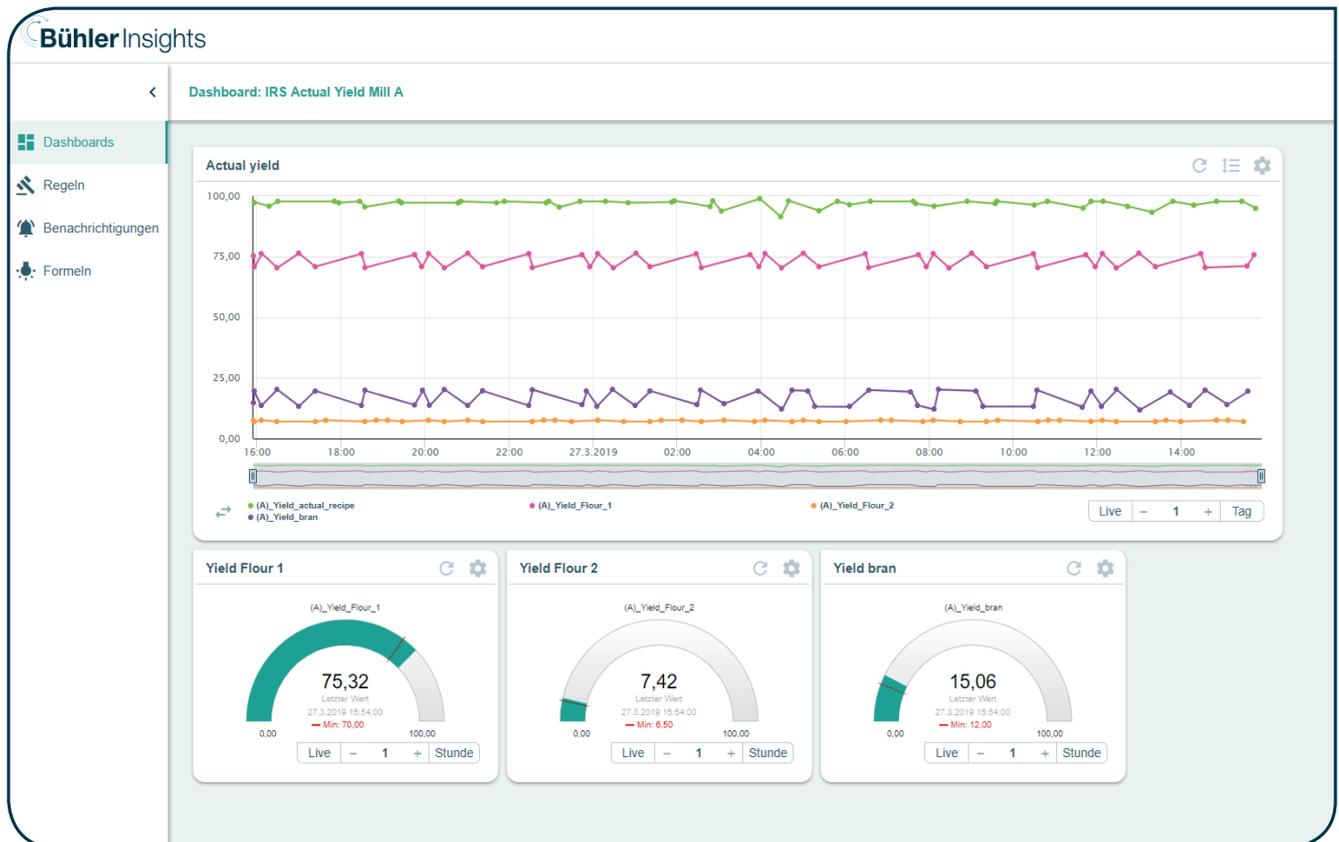
Bühler's YMS integrates data from defined scales directly into Bühler Insights, independent of the plant control system. Visualize and compare various lines against one each other. Thanks to the online data collection even those of plants in different locations. Keep track of recipe based yields over time to improve your overall mill performance.
