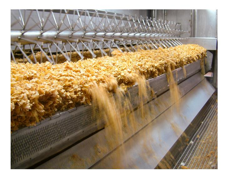
For extruded, flaked and direct expanded cereal applications, the multi-pass conveyor dryer is an ideal solution. The Aero-Dry uses zoned temperature control and alternating airflow to customize the thermal process and maximize the efficiency of heat/mass transfer, ensuring consistent product characteristics across the entire conveyor bed.
