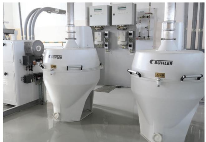
The Bühler dehuller: high throughput capacity and high oat dehulling degree.
