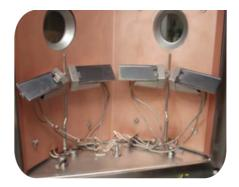
Planetary Systems for extreme concave and convex substrates
