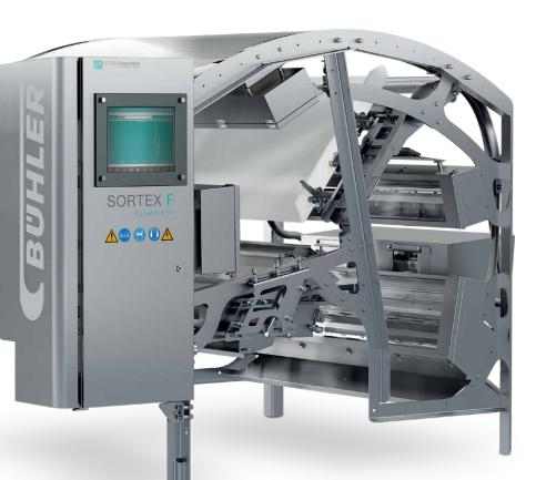
Cleaning the machine is easy thanks to the open and accessible design of the stainless steel frame and sloped surfaces.
