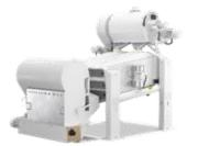
Separator and air-recycling aspiration channel with air-recycling aspiration
