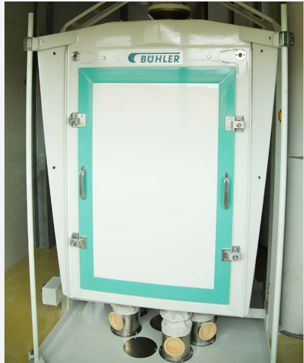
The new small plansifter MPAU is applied for coarse and mealy products in wheat, rye, corn/maize and durum mills for rescreening directly after the mill or before bagging
