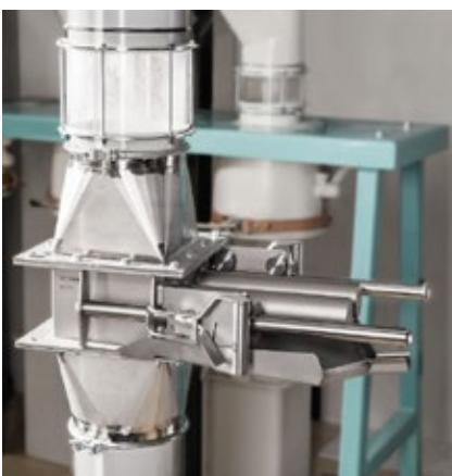
For removing magnetic metal particles from flour, semolina or flakes.
